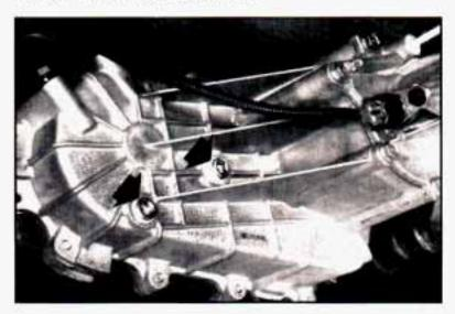
If the level is below the bottom of the filler plug hole, you'll need to add some lubricant. Add enough lubricant to raise the level to the bottom of the filler plug hole.
